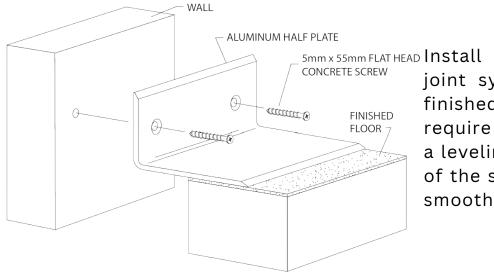
Install the architectural joint system on a leveled, finished floor. This may require grinding or applying a leveling compound on top of the substrate to create a smooth mounting surface
